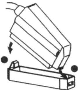
The lamp plug is locked using a mechanical catch. To do this, insert the plug into the flash socket **15**, slightly tilted forward, and then press it tightly into the catch at the rear near the cable duct.
