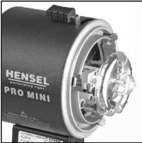
First remove the ignition cable by disconnecting the plug. Wait until the flash tube has cooled down and then remove the glass dome carefully from the head by pulling it out of the spring mechanism (see page 31) and moving it straight away from the head *without touching modeling lamp or flash tube (danger!)*.
