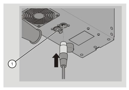
To remove the DMX plug from the device, proceed as follows:
